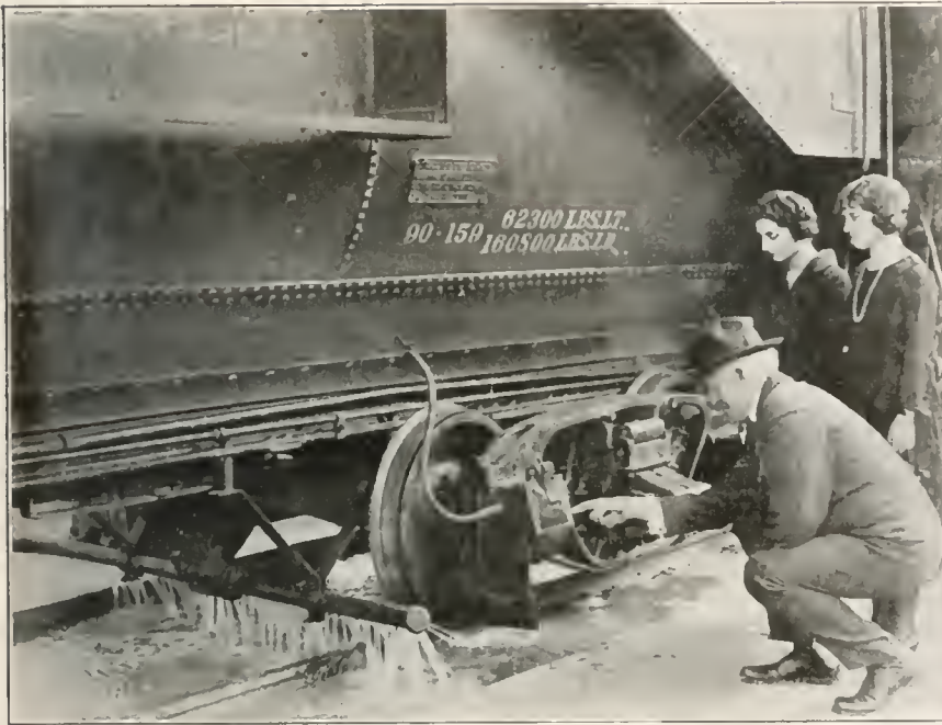
An attachment to the locomotive tender used in sprinkling the roadbed with water keeps down the dust. Many miles of roadbed are oiled for the same purpose and the locomotives of this line burn oil thus eliminating in great measure dust and cinders.
